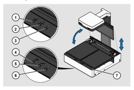
The control panel keys of the Bookeye® 5 V1A can be used to additionally control, program or interrupt the travel of the glass plate during a scanning process.
