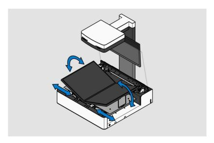
The V position is recommended for very delicate, old books and documents. The opening angle between the book cradle plates is 140 degrees. When the book rockers are lifted into the "V" position, they are held by a support leg on each side. In the "V" position, the plates can also be pushed apart horizontally. The small opening angle puts only minimal strain on the book binding.
