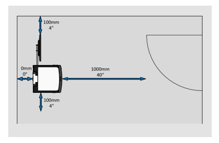
Place the scanner on a level and stable base (at least four table legs). The load-bearing capacity of the base must be suitable for the weight of the scanner (at least 120 kg. / 265 lbs). The dimensions of the base must be suitable for the footprint of the scanner (at least 90 cm x 180 cm /  $36 \times 71$  inch).
