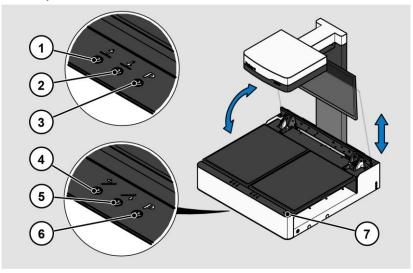
The control panel of the Bookeye  $^{\$}$  5 V1A has seven keys with additional functions for glass plate control.
